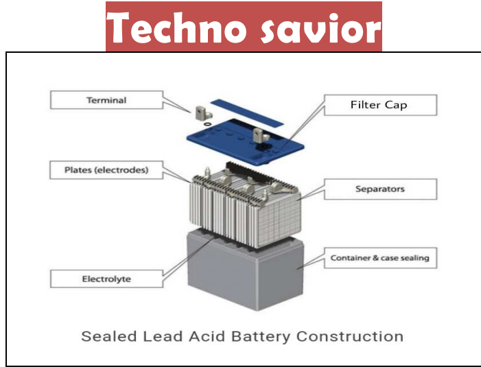
Lead Acid Battery (Source)
